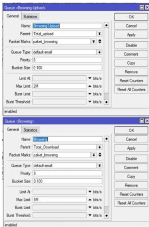
Gambar 10. Konfig Bandwidth Queue Tree Browsing Download Dan Upload
